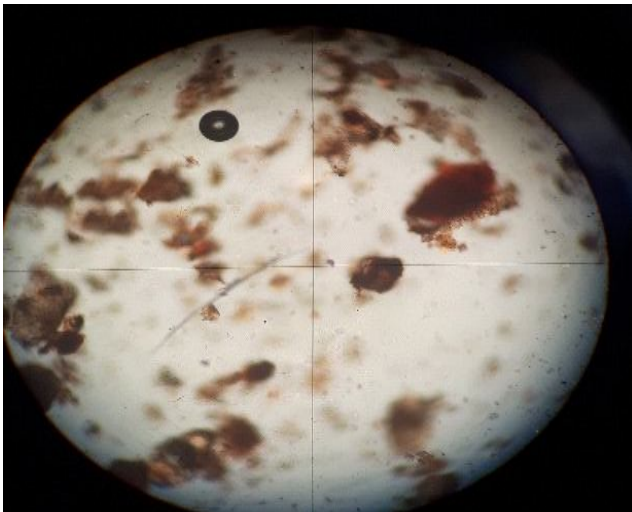
Fig. 5: The edges of chrysotile fibers can hardly be seen in plane polarized light. Taken with 100X magnification power.
