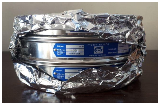
Fig. 3: Sieves arranged sequentially from top to bottom (2.3 mm, 300 \mu m, 75 \mu m)
