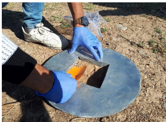
Fig. 2: Collection of surface samples.
